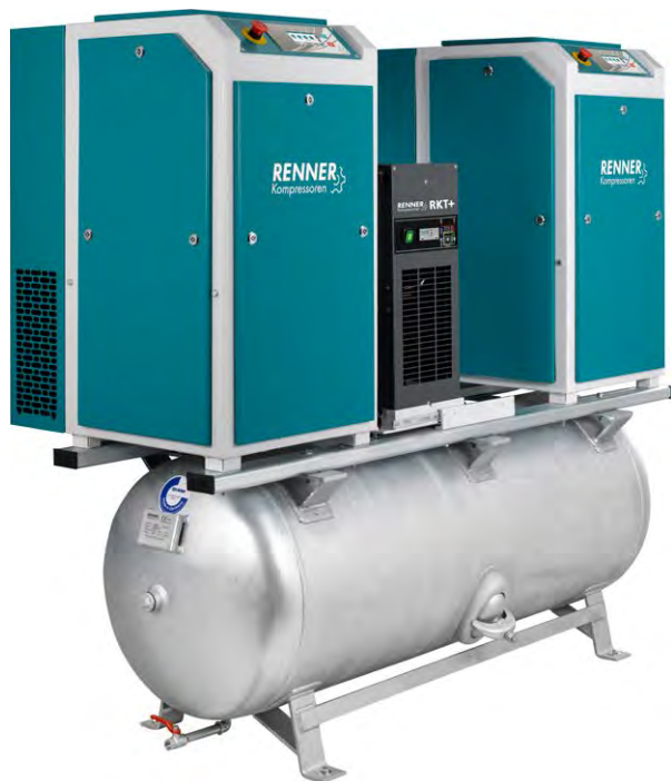
RSDKM-PRO multiple unit with two configurable compressors of the RS-PRO series on galvanized 500 ltr air receiver, with refrigeration dryer RKT+ and electronic control RENNERtronic Touch.
